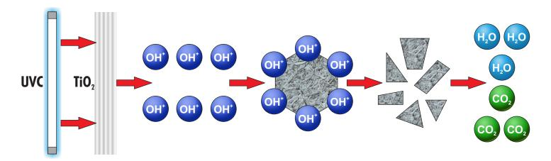
Photocatalyst (TiO<sub>2</sub>) Absorbs UVC Light (254 nm) Oxidizing Hydroxyl Radicals Formed
